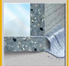
**No profile** Water flows through the construction joint
