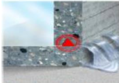
Hydrophilic gasket in joint – water ingress reducing
