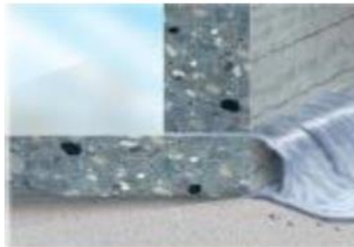
No joint – water ingress
