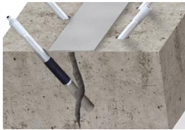
Drill packer hole through the crack
